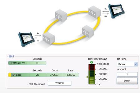
The MAX-880 offers the ability to preconfigure bit-error-rate (BER) thresholds that are user-defined prior to running the test, thereby generating a simple pass/fail verdict at the conclusion of test to overcome misinterpretation of test results.
