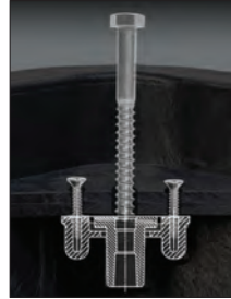
Non-Seizing Bolt System Allows Field Replacement
